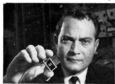
OPTICAL MEMORY ELEMENT developed at Sandia is shown framed in an integrated circuit flat-pack mount held by co-inventor Cecil E. Land (5143). The one-quarter-inch by one-fifth-inch prototype model can store over five times as much information in a given space than those common to most computer memories.
